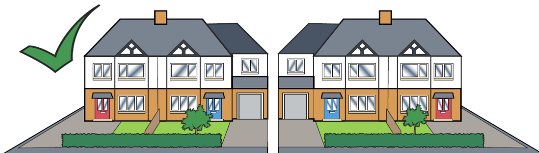
Figure 9a Acceptable side extension
