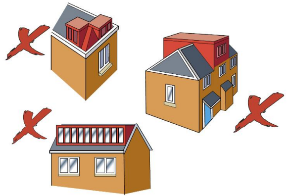
Figure 14 Unacceptable dormer extensions
