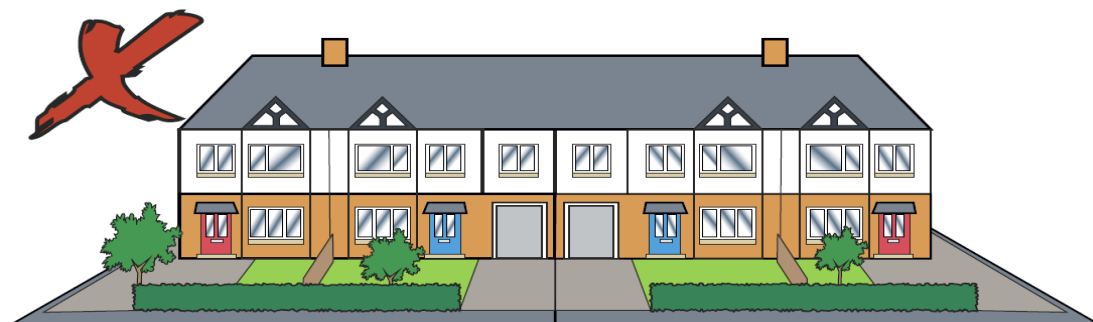
Figure 9b Unacceptable side extension
