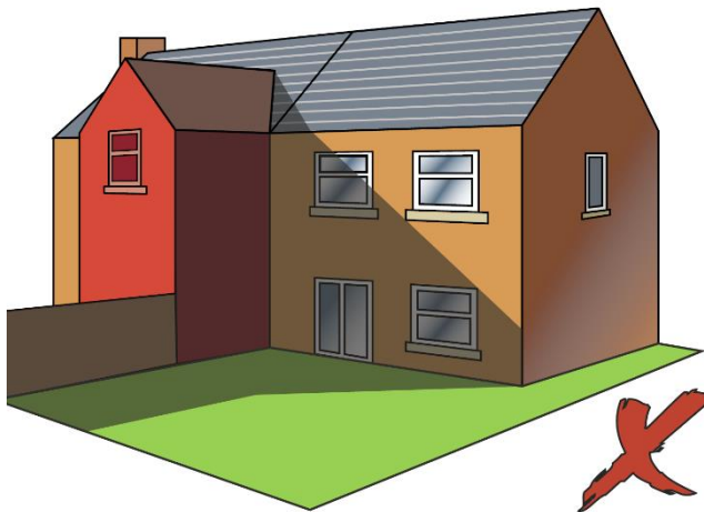
Figure 3a Unacceptable overshadowing
